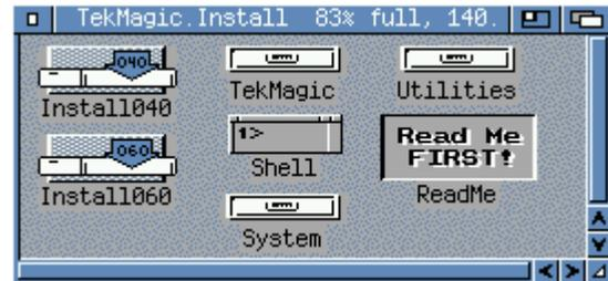
It should be noted that there are four programs needed by the 68040 processor to insure maximum performance. These are: **CPU**, **Setpatch**, **68040.library**, and **KSRemap**. The latest of all four programs are included on the Install disk and these can be automatically installed if selected by the user. Only one of these programs, "KSRemap" is supplied by TekMagic; the rest are standard Amiga programs.
